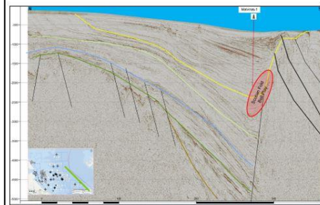
Figure 2.4.4: Schematic distribution on NS seismic line of the main exploration plays in Malvinas Basin
